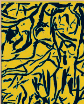
Photomicrograph of Grey Cast Iron (100X) showing carbon in the form of graphite flakes.
